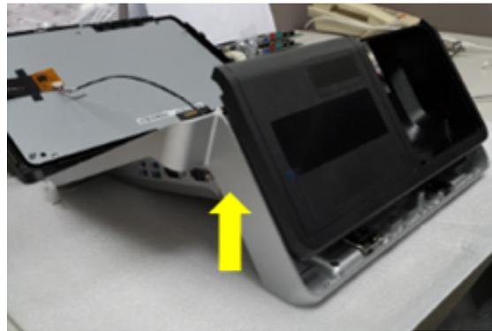
10. Loosen 4 screws, disconnect the cable and then take out the VFD.
