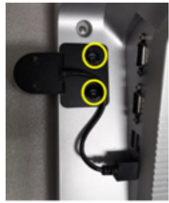
2. Plug the USB cable of the MSR/i-Button into the side USB port
