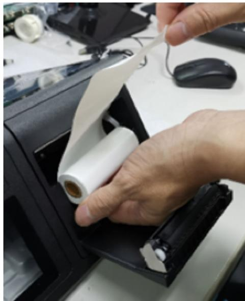
4. Remove excess paper in the direction of the printer.
