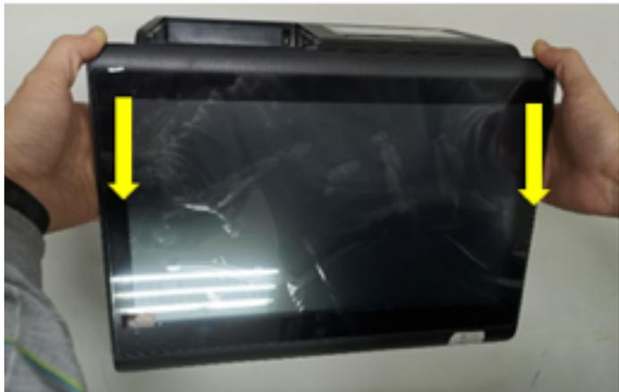
3. Push the lock slider down to unlock the printer cover button
