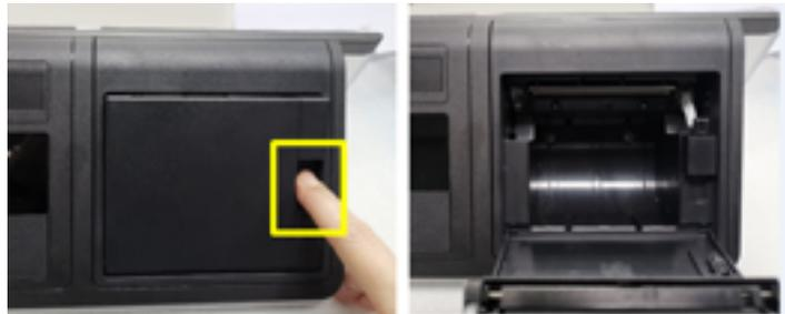
3. Insert the paper in the correct direction of the roll paper
