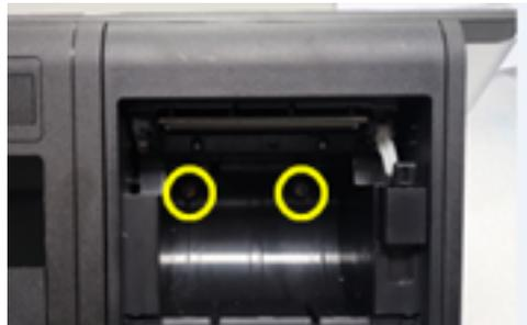
4. Pull out the printer module
