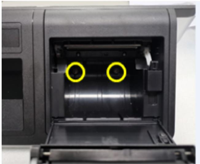
6. Pull out the printer module
