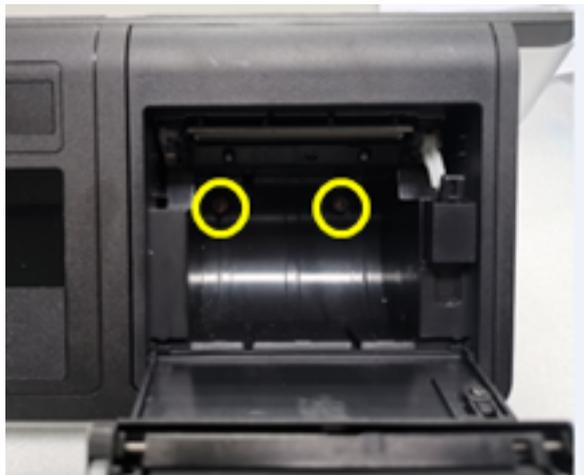
6. Pull out the printer module
